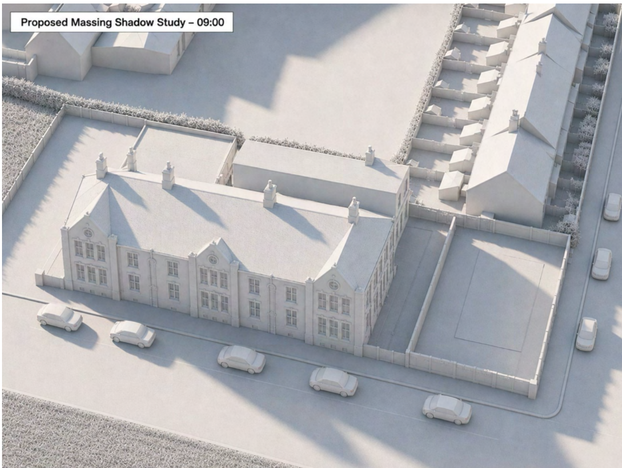
Figure 5: Proposed massing shadow study at 09:00. Morning shadows are naturally longer than midday shadows and should be compared against the existing urban condition.
