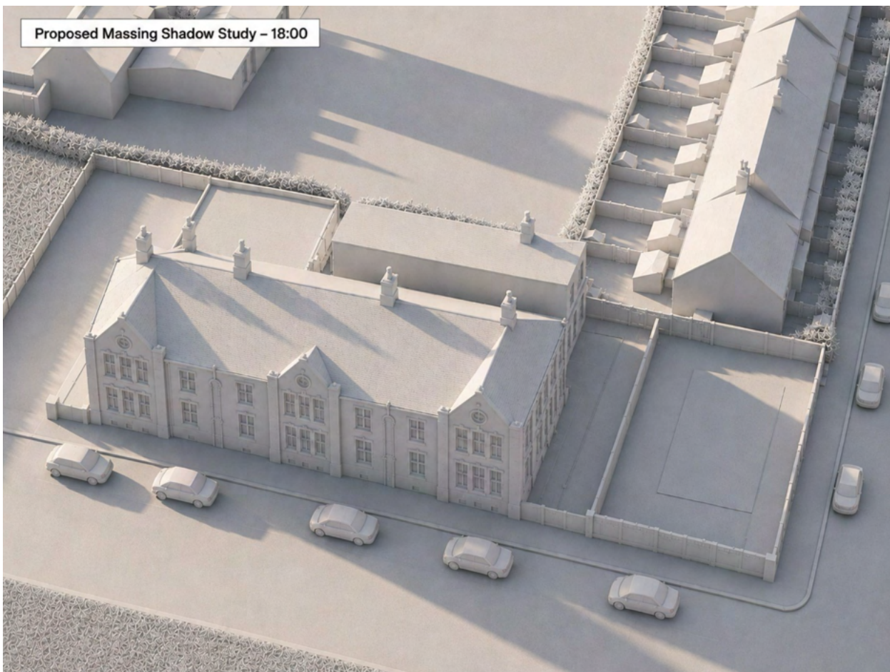
Figure 8: Proposed massing shadow study at 18:00. This condition is most relevant during late spring and summer when daylight remains available into the evening.
