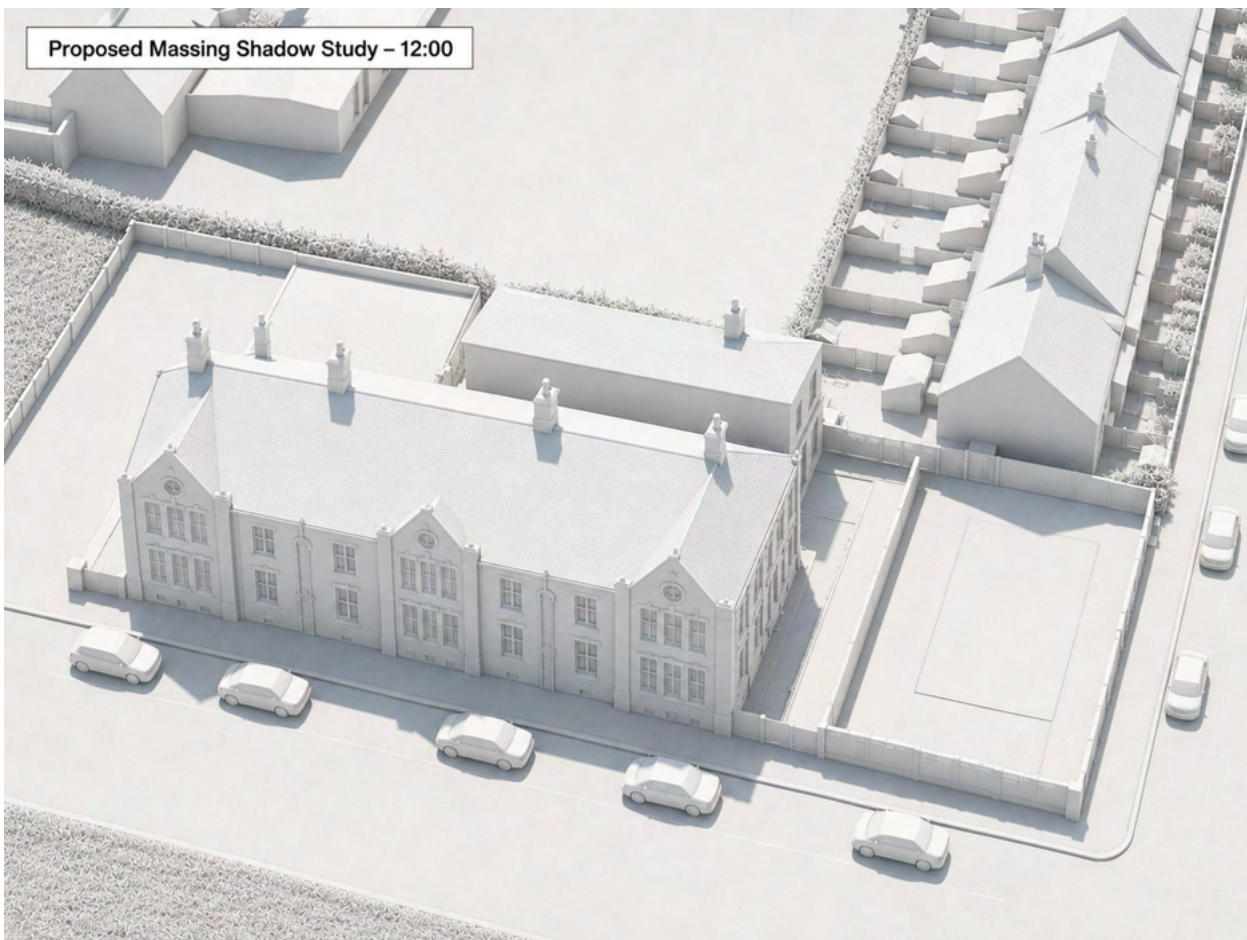
Figure 6: Proposed massing shadow study at 12:00. This represents the period when the sun is highest and shadows are typically shortest.
